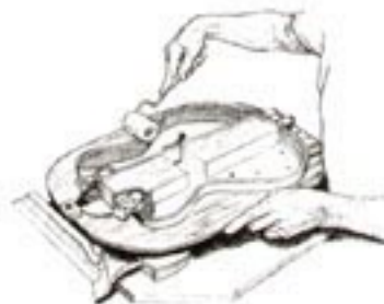
Hand application of top & bottom to rims
