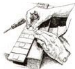
Installation of fingerboard inlays
