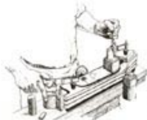
Hand guiding through router in shaping the neck
