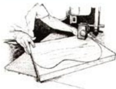
Band saw cutting body shape.
