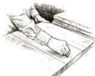
Matching wood panels for grain and color
