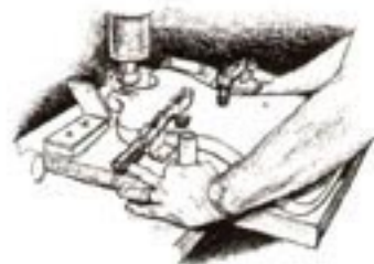
Routing solid body for neckpiece
