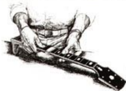
Fret board positioning and installation
