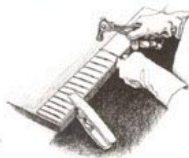
Installation of frets into neck
