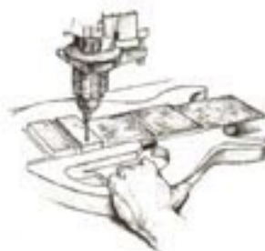
Drilling holes for anchoring strings through the body
