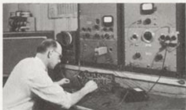
A Gibson engineer is analyzing changes in power output. Complete modern test equipment includes oscillators, voltmeters, analyzers and oscilloscopes to check amplifier performance.
