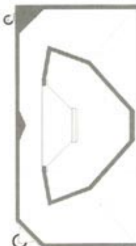
Exclusive folded horn, sealed enclosure tuned to resonate all bass frequency at equal volume. 18" extremely heavy duty speaker acoustically matched to enclosure.
