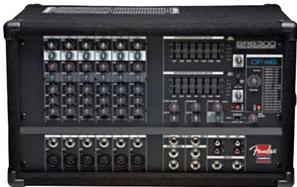
The SR6300 mixer is designed for performance! The SR6300 features six input channels, 300 watt power amp, dual seven-band graphic EQ, 16 selectable digital effects and 48 volt phantom power. The ultra clean power amp works in left/right, main/monitor and in bridged modes.
