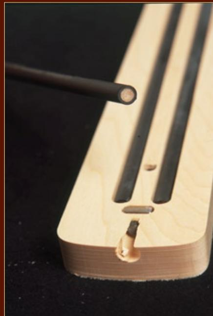
Neck warping is a bass player's worst nightmare. With Fender's Posiflex neck support, two rods are placed in the neck just beneath the fingerboard on either side of the truss rod. The truss rod functions for normal neck adjustment but much smoother and more accurately over the length of the neck, eliminating any "humps, bumps and curves" – just one smooth continuous curve. The stability over time and under various climatic conditions is unparalleled when compared to normal wood construction.
