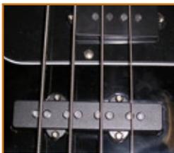
*"Before too long I realized that to be able to get the harmonics to jump out (like Jaco), I needed to install a Jazz Bass-style bridge pickup. Additionally, I decided upon an ebony fingerboard and figured the easiest and least intrusive way to switch between the pickups was to use a three-position Fender® Stratocaster® switch.*
