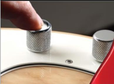
Press the S-1 switch and the split single-coil pickup of the American Series bass guitar goes from series to parallel, giving the bass a brighter, snappier tone with more midrange bite and treble snap.
