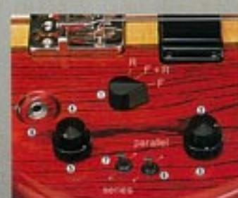
The single shaft, twin-pot control of SB800
