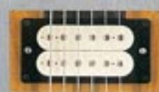
The X80 is fitted with the renowned DiMarzio dual-sound humbuckers; a series/parallel selector switch provides the usual humbucking sound or a more attacking sound without loss of humbucking effects.
